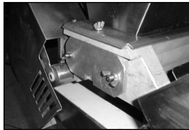
Template correctly fitted in hopper
