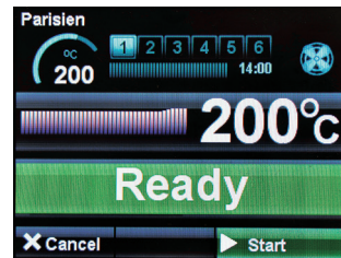
When the oven reaches the correct temperature the ready screen will show.
