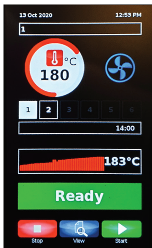
When the oven is at the desired temperature the ready screen will be displayed.
