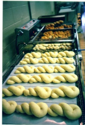
Above: Mark VI Feed Table with 'Twist' donuts. The Mark VI can accommodate almost any size and shape of donut.
