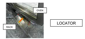
Using the push-pull tool, push the cassette into the oven as far as it will go.
