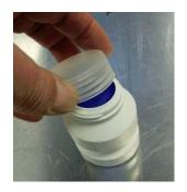
Unscrew and remove the protection cap. Do not try to puncture the wax plug.
