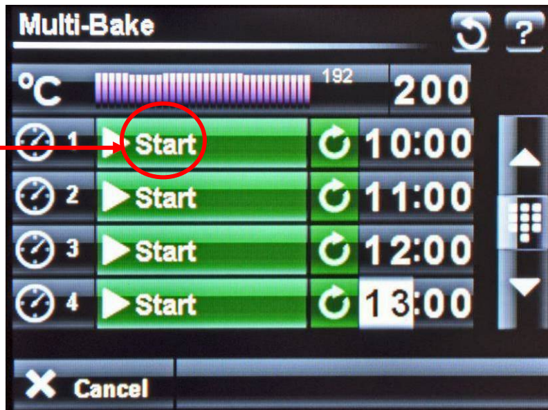
MULTI-BAKE SETUP SCREEN SHOWING FOUR TIMERS SET
