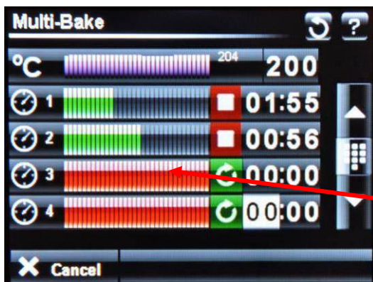
MULTI-BAKE SETUP SCREEN WITH FOUR TIMERS RUNNING
