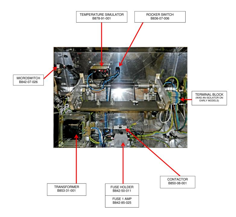
VIEWED FROM REAR WITH DOOR OPEN. DISCONNECT FROM MAIN POWER SUPPLY BEFORE OPENING.
