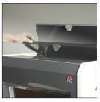
Rear safety cover Closing it initiates the slicing process and it opens automatically when slicing is complete.
