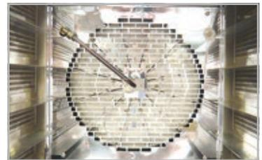
Fully welded stainless steel chamber with integrated steam system
