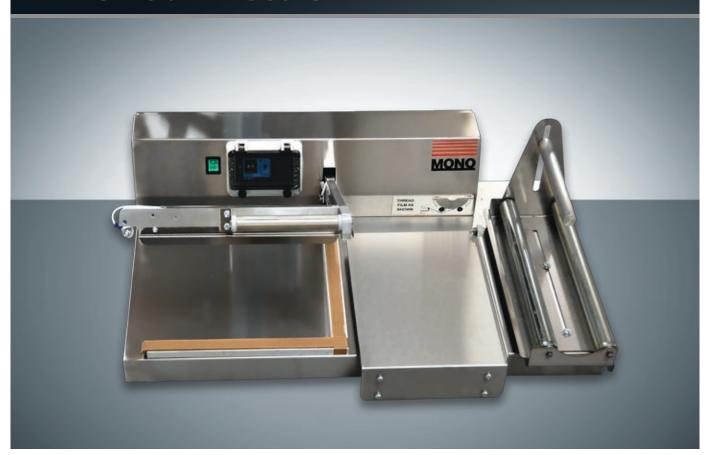
MONO Equipment's compact Robin L-Sealer has a maximum seal area of 28cm by 28cm and can quickly and easily seal approximately 700 products per hour.
