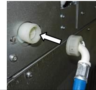
OVEN WATER CONNECTION AT REAR
