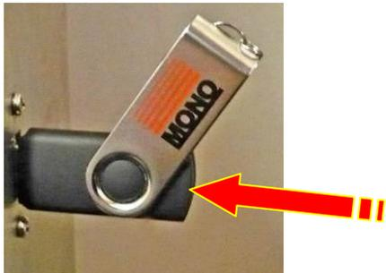
Insert the USB memory stick into the socket on the oven panel. (Rubber plug may have to be removed first).
