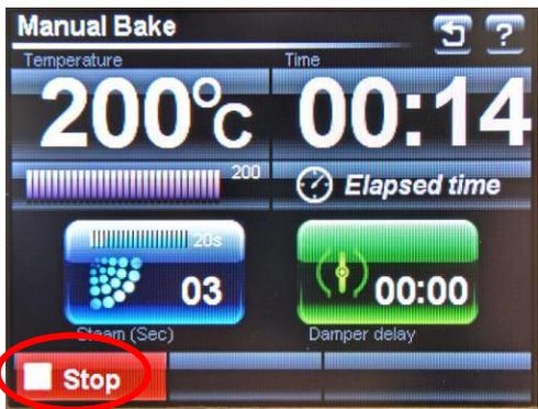
TOUCH "STOP" WHEN END OF BAKE BUZZER SOUNDS OR WHEN REQUIRED IF NO TIME WAS ENTERED
