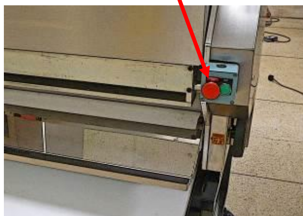
TO STOP MOULDER EMERGENCY STOP BUTTON
