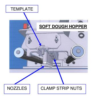
4 To reduce weight and bulk, separate and remove empty feed hopper from pump assembly whilst still on the machine by unscrewing the wing nuts.
