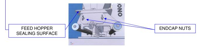
7. Withdraw the end-cap with the pump gears.
