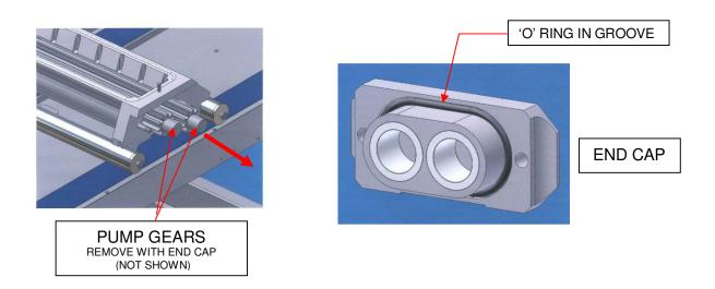
4. Remove remainder of pump assembly from the machine and remove remaining end-cap to fully dismantle pump assembly components for cleaning.
