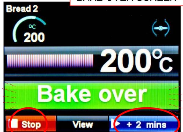
AT THE END OF THE BAKE TIME A SOUNDER WILL BE HEARD AND "BAKE OVER" WILL FLASH. TOUCH "**STOP**" AND OPEN THE DOOR TO REMOVE THE PRODUCT.
