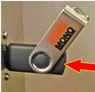
Insert the USB memory stick into the socket on the oven panel. (Rubber plug may have to be removed first).
