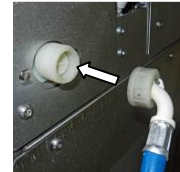
OVEN WATER CONNECTION AT REAR
