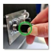
FIRSTLY: ALWAYS ensure the flat side of the connector, with the arrow symbol, is facing to the left, when connecting the power supply.
