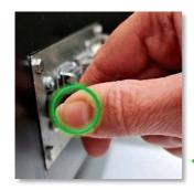
ALWAYS: Grip the flat area of the connector between thumb and finger and pull gently to remove the power supply.
