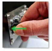
STEP 1: Holding the flat side of the connector between finger and thumb, push until the silver part of the connector is no longer visible.
