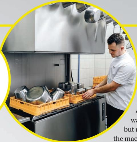
and marketing manager, Wexiödisk, the WD-12S is a game-changer partly because the compartment size has been widened. “We can do the 500mm by 500mm wash baskets as previously, but now we’re also able to load the machine with three plastic boxes used for transporting food and other items that are 600mm by 400mm. We have been able to take this machine to another level and improve many things.”
