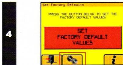
Press the **SET FACTORY DEFAULTS BUTTON**. Then press The **COGS** Button to enter the System Menu.
