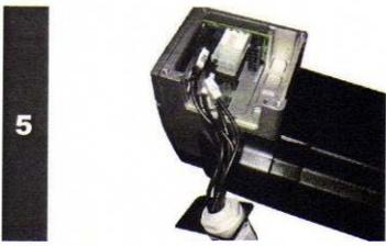
Slide the cable gland plate from the motor housing to gain access to the connectors.
