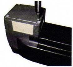
Re-fit the motor control box lid for each motor (ensure that the earth cable is connected).
