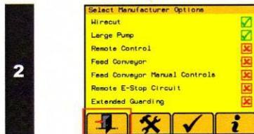
Select the options installed on your machine. Press the exit button.
