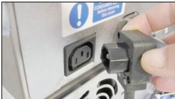
Figure 45: Plugging in the condenser unit
