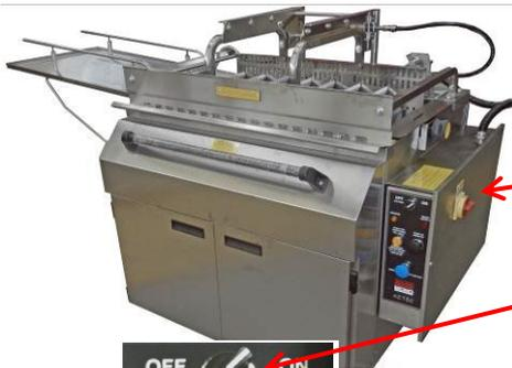
1. Mains power connected? (Check socket on wall or store isolator)
