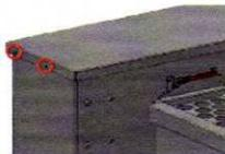
Remove the 4 screws securing the main enclosure lid (2 on each side) using 1 4mm allen key and 10mm spanner/socket to gain access to the electrical control panel. To remove the lid lift the lid at the front and slide to the rear then lift to remove.
