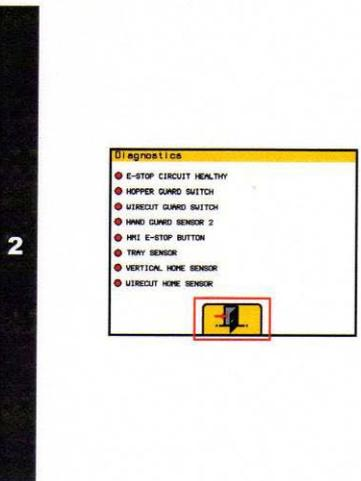
Test that **ALL** inputs are working correctly using the diagnostics page.
