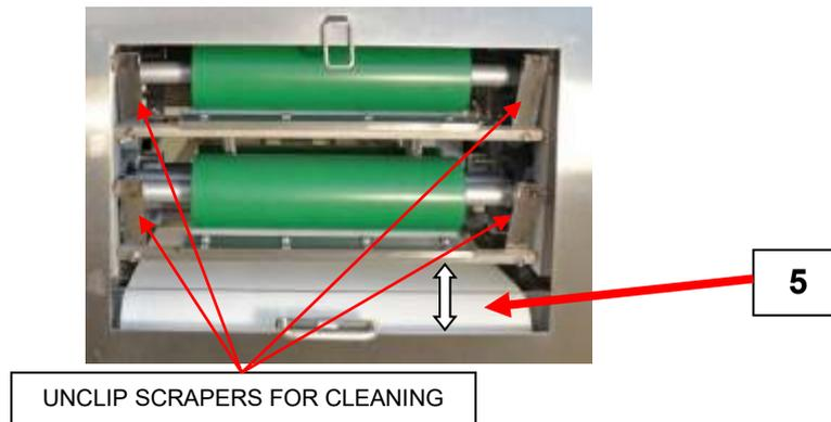
12. Unclip and wipe the rear scrapers
