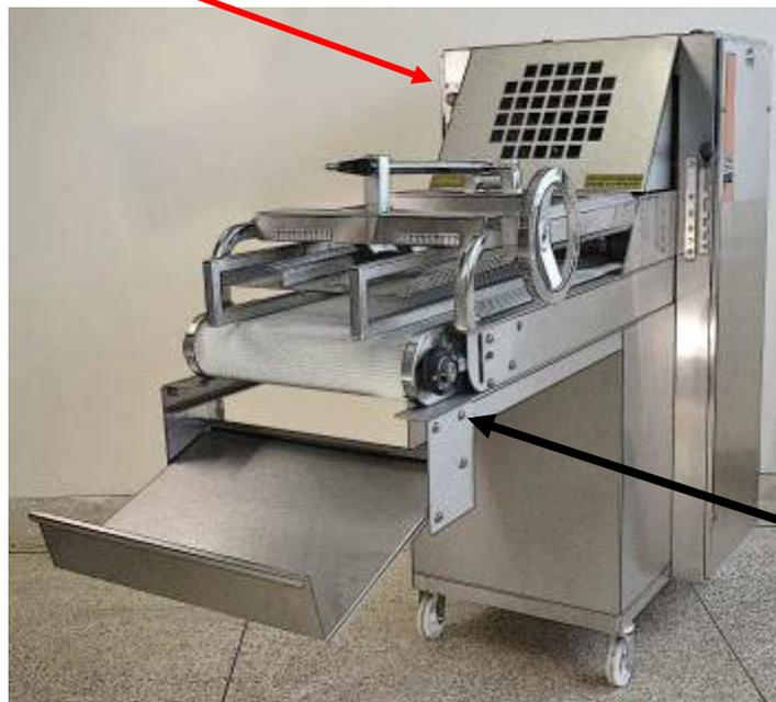
If used with a prover always start the moulder before the prover or a build-up of dough could clog the moulder hopper.
