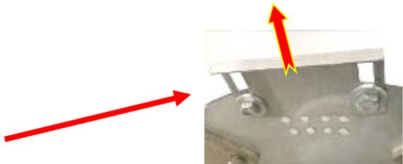
MOVE DUSTER CONTROL PLATES TO CONTROL THE FLOUR IN THE AREA REQUIRED. THE MORE HOLES SHOWING, THE MORE FLOUR FLOWS.
