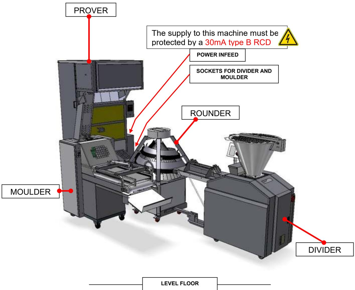
1. The plant should be positioned on a solid level floor.
