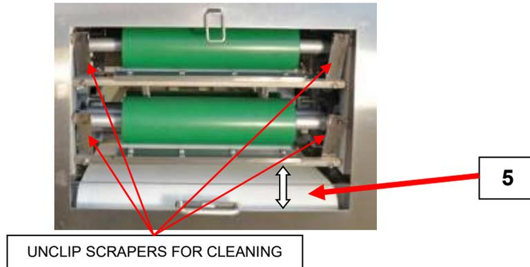
12. Unclip and wipe the rear scrapers
