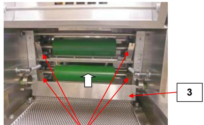
UNCLIP SCRAPERS FOR CLEANING
