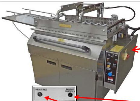
1. Mains power connected? (Check socket on wall or store isolator)
