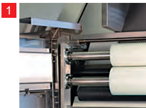
Cleaning The easily accessible door allows for easy cleaning of the rollers, scraper and curling chain.
