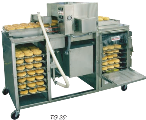
TG 25: Less than 5 minutes start-to-finish. 25 dozen/hour typical rate overall.
