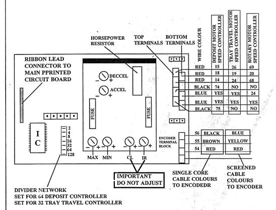
A) Set appropriate speed setting display to "00", then adjust "MIN" potentiometer to indicate a motor minimum speed setting, clockwise to increase speed, and anticlockwise to decrease speed.
