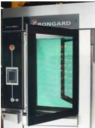
Magnets allow the external window to open easily
