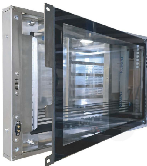
Figure 5.2: Inner glass panel moved away from the door
