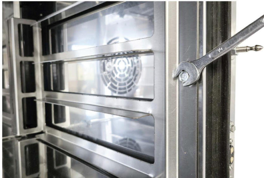
Figure 5.3: Unlocking the tray runners
