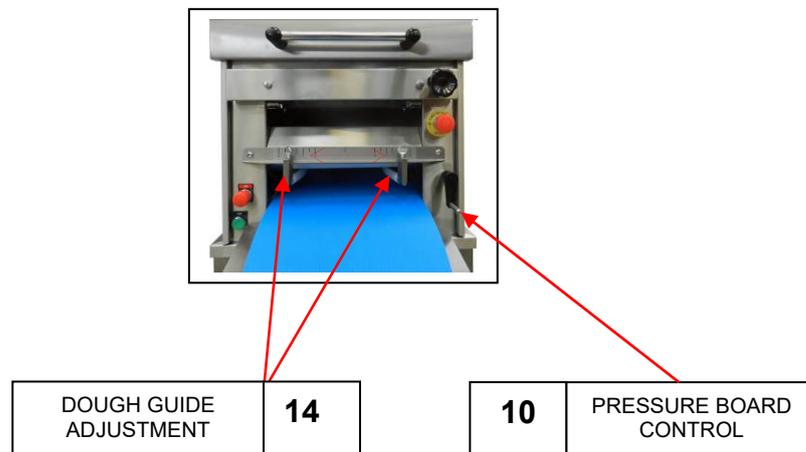
The pressure board dough guides (14) are adjusted by means of the guide clamps. The length of the dough piece required determines the width at which the dough guides are set. It should be noted that the dough guides and pressure board adjustments are relative to each other and should be adjusted accordingly.
