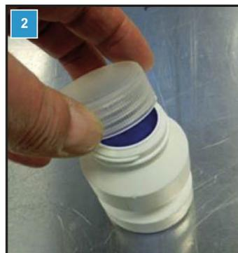
9. Screw the cartridge face down into the locator hole, firmly.
