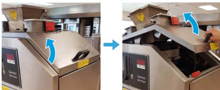
Figure 9.2: Lifting the outer access door upwards
