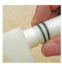
SLIDE RING DOWN TO SECOND GROOVE, PASSING OVER FIRST RING
