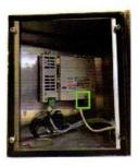
Connect the HMI cable to the connector marked ETHERNET. Ensure that the cable is pushed in firmly, you should hear a "click".
