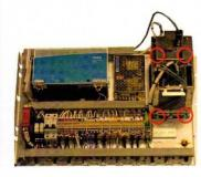
Remove 4x screws using a posidrive screwdriver and remove TLCC motion controller.
