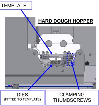
4 To reduce weight and bulk, separate and remove empty feed hopper from pump assembly, whilst still on the machine, by unscrewing the wing nuts.
