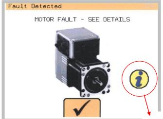
PRESS THIS BUTTON IF MORE INFORMATION IS REQUIRED AS TO WHICH MOTOR IS AT FAULT
