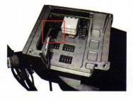
Do NOT remove the STOP connector, this cable can be moved out of the way to gain access to the switches.
