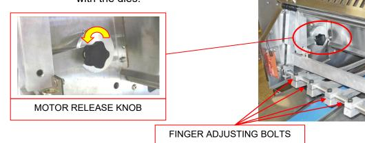
5. Adjust individual finger bolts to raise the wire to touch the bottom surface of the dies used in the template.
