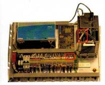
Remove the 2x 'D' connectors from the TLCC using a small screwdriver. Remove the trunking lids. Trace the wires back to the terminals (C1+ / C1- / C2+ / C2-) and remove using a small screwdriver.
