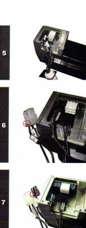
Slide the cable gland plate from the motor housing to gain access to the connectors.
