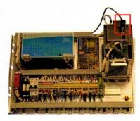
Remove the 'D' connector from the TLCC using a small screwdriver.
