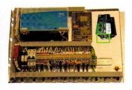
Connect the power supply plug to the M251 (connector at bottom).
