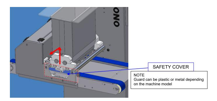
Slacken template clamp strip nuts or thumbscrews (depending on type of hopper).
