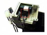
Carefully remove the POWER connector, pull to remove (long nosed pliers can be used).
