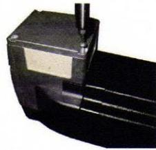
Re-fit the motor control box lid for each motor (ensure that the earth cable is connected).
