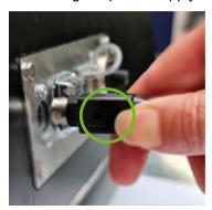
**b.** Holding the flat side of the connector between finger and thumb, push until the silver part of the connector is no longer visible.
