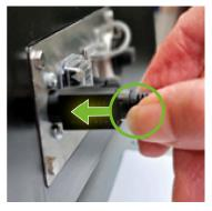
When unplugging, grip the flat area of the connector between thumb and finger and pull gently to remove the power supply. Never pull when holding any other part of the cable.
