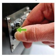
**c.** Grip the power-lead immediately behind the flat area of the connector and push forwards until you feel or hear a click.
