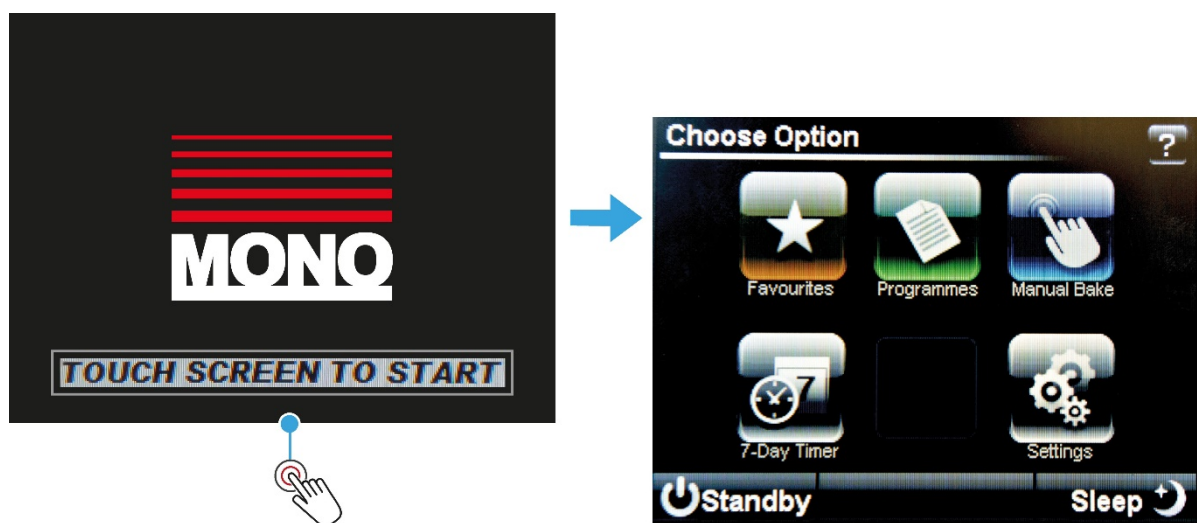
Figure 5.5: Exiting Standby mode
