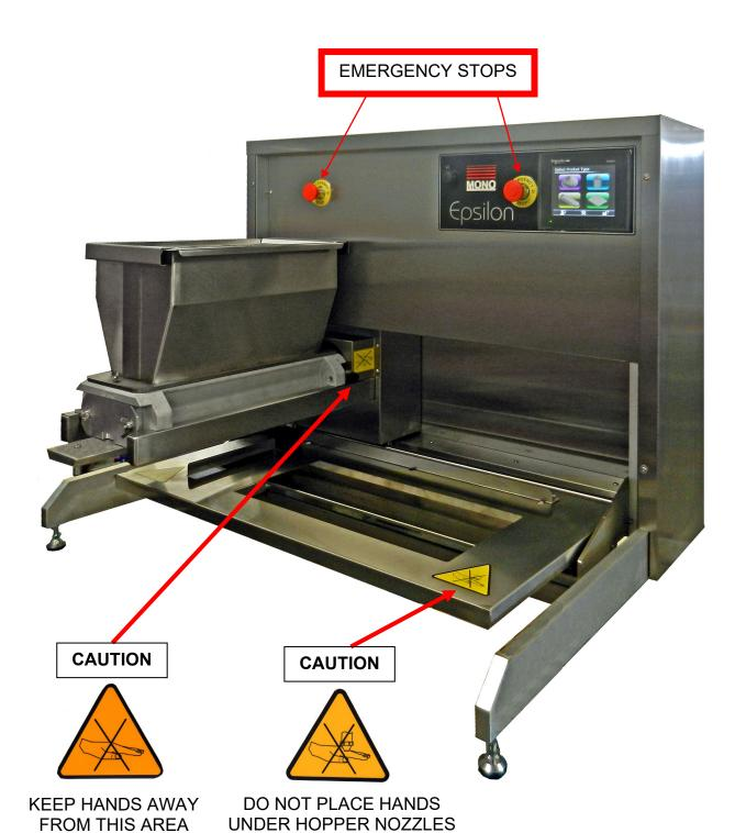
ALL OPERATIONS ARE ACTIVATED BY TOUCHING AREAS ON THE SCREEN WITH A FINGER. DO NOT USE EXCESSIVE FORCE OR HARD OBJECTS AS THIS WILL INVALIDATE MACHINE WARRANTY.
