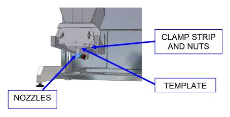
3 To reduce weight and bulk, separate and remove the empty feed hopper from the pump assembly, by unscrewing the wing nuts, whilst still on the machine.
