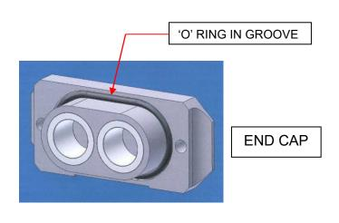
4. To fully dismantle pump assembly components for cleaning, remove remainder of pump assembly from the machine and remove remaining end-cap.
