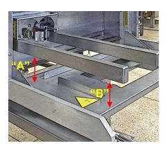
If not the same, an adjustment can be made by raising or lowering the adjusters under the table. There is one each side to allow the table to be adjusted evenly.
