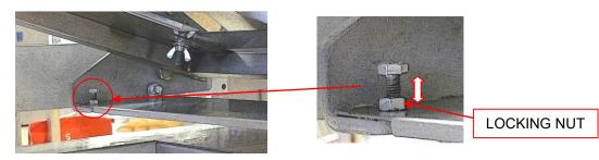
Lift the front edge of the table and, with a suitable spanner, release the locking nut. Screw the adjuster bolt up or down and then lock it in position with the locking nut.
