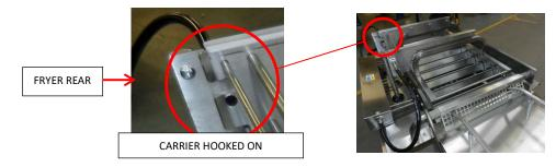
• Screws at bottom of carrier have been tightened. (Unlikely but should be loose to allow up/down movement).
