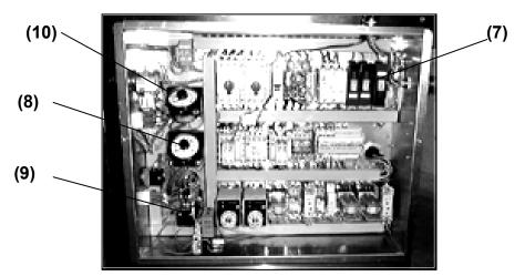
**NOTE:** WHILST COVER (6) IS OFF, CHECK THAT THE THREE THERMOSTATS ARE SET CORRECTLY.
