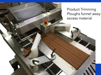
Clean Scraping Precision scraper design removes all product from rollers ensuring material moves cleanly through the SlabLine.
