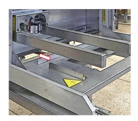
This allows different width trays to be accommodated. To adjust the position of the back guide, remove the table and turn it over. Loosen the thumb nuts and slide the sheet across to the desired position. Tighten the nuts and replace the table.
