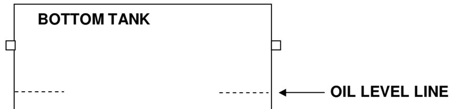
**Do not mix different makes or types of frying oil** as a reaction can result in a thick flour-like sediment forming in the lower tank which can block the filtering system.
