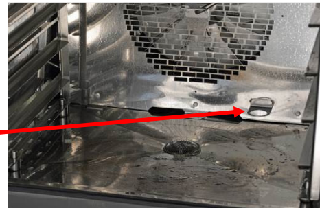
Locator hole on the rack-cassette
