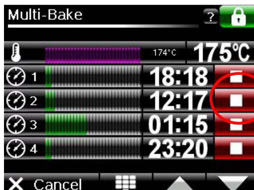
MULTI-BAKE SETUP SCREEN WITH FOUR TIMERS RUNNING
