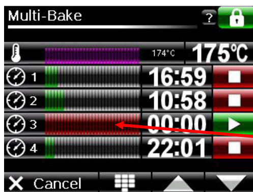
MULTI-BAKE SETUP SCREEN WITH FOUR TIMERS RUNNING
