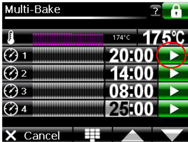
MULTI-BAKE SETUP SCREEN SHOWING FOUR TIMERS SET
