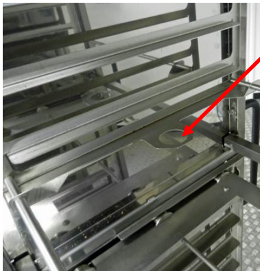
Locator hole on the rack-cassette
