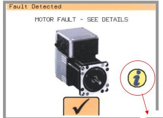
PRESS THIS BUTTON IF MORE INFORMATION IS REQUIRED AS TO WHICH MOTOR IS AT FAULT
