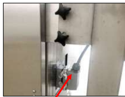
Connect the Roll Forming Unit Power Supply to the Socket on the Two-Pocket Roll Plant and Clip in Place
