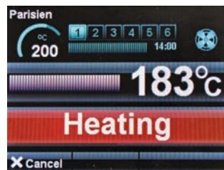
The heating screen shows the temperature progress.
