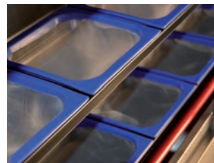
The polyethylene pockets are perforated to allow air to circulate to prevent sticking.
