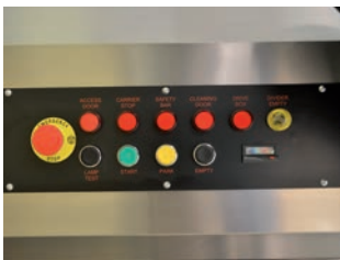
The easy to reach control panel features an integrated dough processing counter to record the number of products produced.
