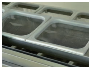
The polyethylene pockets are perforated to allow air to circulate around the dough and to prevent sticking.
