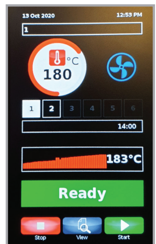
When the oven is at the correct temperature the ready screen will show.
