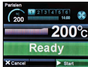
When the oven reaches the correct temperature the ready screen will show.
